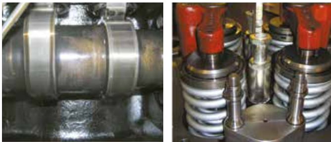
Figure 4 (left). Engine inspections during field trials reveal a clean camshaft in a Pielstick engine after 5,000 hours of operation under severe conditions with Shell Argina X (left). No deposits were observed on the valve deck of a Wärtsilä 64 engine after 5,000 hours of operation with Shell Argina XL (right).
