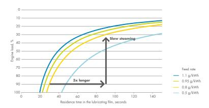
THREE TIMES LONGER: Plotting oil residence time against engine load for a fixed feed rate shows that slow steaming may force the oil to work for three times longer than at normal steaming speeds.
