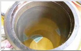
**EXTRA PROTECTION:** A GE-J 312 gas engine burned landfill gas for 35,000 hours, and Shell Mysella S3 S helped to provide ring-belt cleanliness and low ring wear (top) and good liner protection (bottom).
