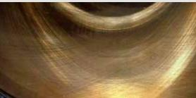
demonstrated excellent ring groove cleanliness (top) and left the cylinder liner in an excellent condition (bottom) in a Wärtsilä 20V34SG engine after 16,000 hours of operation without an oil change.
