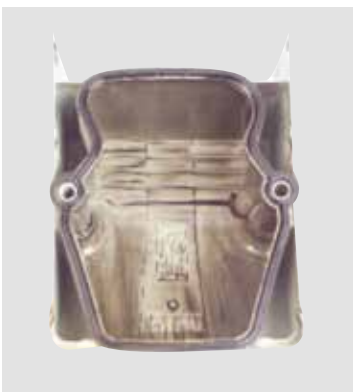
Rocker cover from Mercedes-Benz engine: excellent cleanliness after 750,000 km on-highway service
