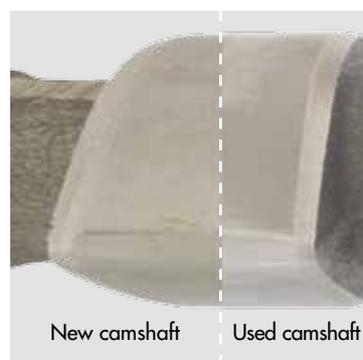
Mercedes-Benz OM-646LA engine test: shows minimal wear after running for 300 h using Shell Rimula R5 LE 10W-30.
