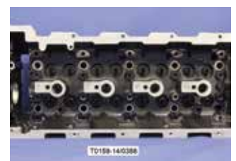
Valve deck (OM 646 LA)
