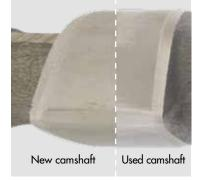
Mercedes-Benz OM-646LA engine test: shows minimal wear after running for 300 h using Shell Rimula R5 LE 10W-30.
