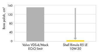
Control of bore polish as measured in the Volvo D-12D engine test.
